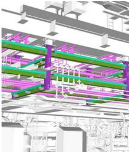
Phase 1: 3D BIM Design - Design for Manufacturing and Assembly – (DMFA)
